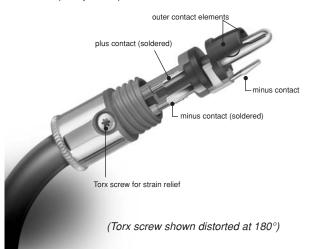
But your nextgen plug WBT-0110 makes it even more comfortable: By pressing the two snap hooks left and right you have the possibility to pull out the whole Central Contact Unit by the front. This way you may solder the plus and the minus outside the connector's body.
